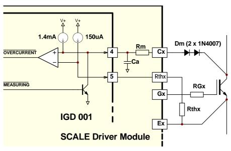
The 2SD106AI-17 dual driver has a collector-sense circuit to protect the power semiconductors. It is shown in Fig. 4
