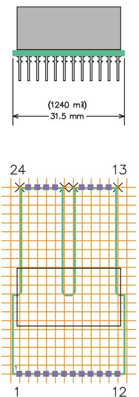
Fig. 3 Front view (top) / Layout overview component side (bottom) 2SD106AI-17
