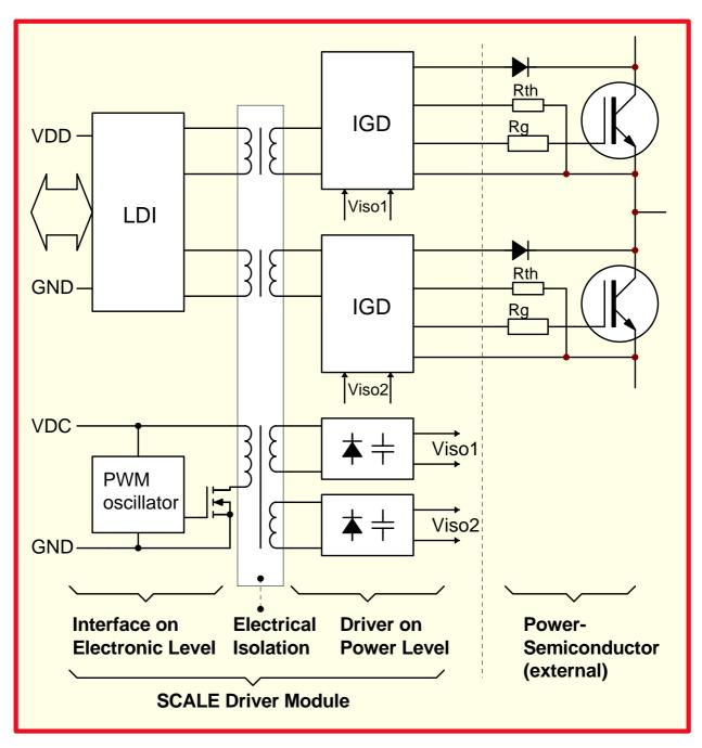
Fig. 1 Block diagram of the 2SD106AI-17
