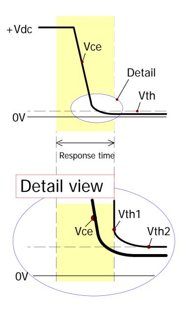
Fig. 5 Collector-sense voltage curve
