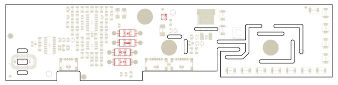
Fig. 2: Assembly drawing of 1SP0335D2S1 with highlighted gate resistors
