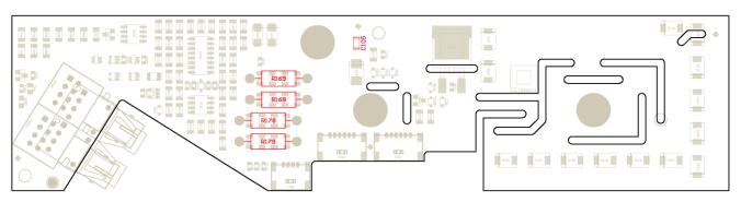
Fig. 1: Assembly drawing of 1SP0335x2M1 with highlighted gate resistors
